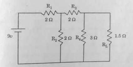
Find the current through the 3  $\Omega$  resistor of the following network using superposition theorem :
